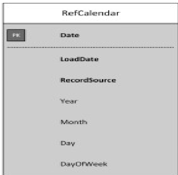
Figure 21: The Figure shows the ER model for reference table ( Physical design )
